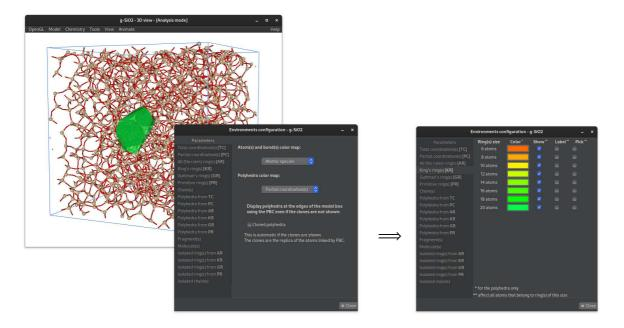
This tab provides interactors with King's ring statistics calculation results: color of the ring's polyhedra, and then options to show/hide, label/unlabel, or select/unselect atom(s) involved in any ring(s) of the corresponding size.
