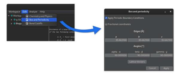
The new model now uses periodic boundary conditions, if required the box can be displayed in the 3D window using the corresponding menu button: "Model -> Box -> Show/Hide".
