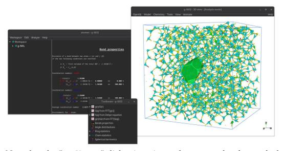
Note that the "Toolboxes" dialog is active and some results, from calculation performed previously and stored in the project file, are available, including for the radial distribution function g(r).
