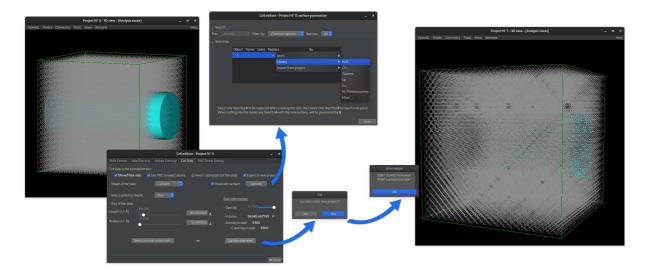
Then just click on "Cut this slab now!" to create a new project, that will contain the new material: a C diamond cell where the atoms inside the cylinder are removed, creating a surface, and where non-bridging bonds have been passivated using  $H_2O$  molecules.
