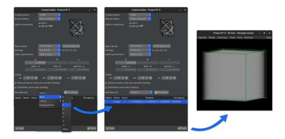
The 3D window is populated with the newly created structure, in this example a  $"20\times20\times20"$  supercell of pure diamond.
