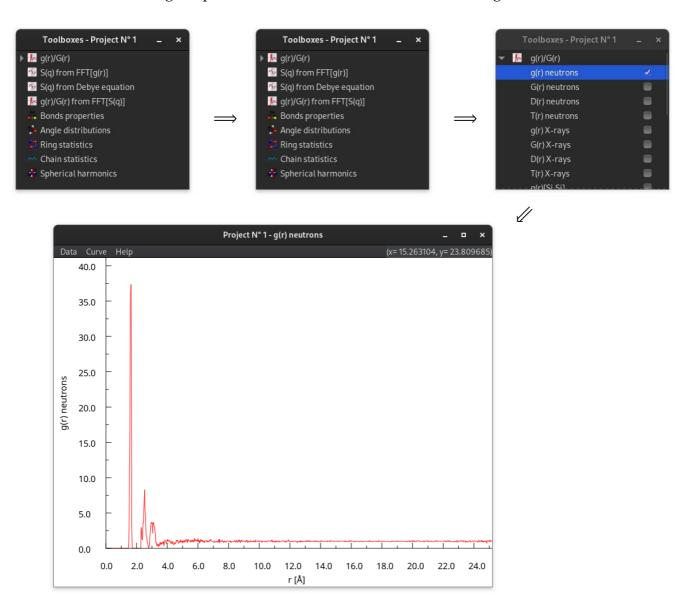
In the "Toolboxes" dialog open the result of the calculation to display the g(r) of the active project, in this case the new model created from the atom selection.
